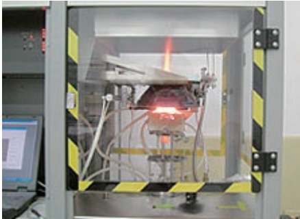
Cone Calorimeter Testing Device (ISO 5660)
