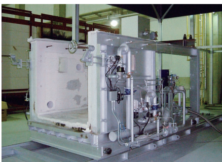
Structural Fire Testing Furnace (Medium scale)
