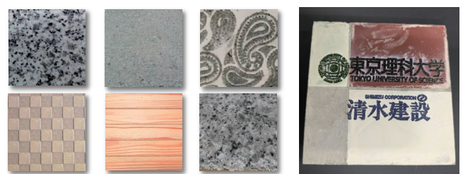
Fig. 4 Various textures achieved using the developed printing technology
