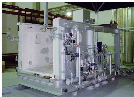
Structural Fire Testing Furnace (Medium scale)
