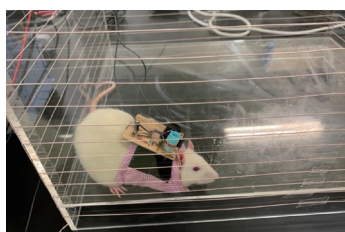
Figure 1 Wireless power transmission to an implantable momentum meter
