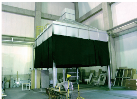
Calorimetry Hoods (5 m × 5 m)
