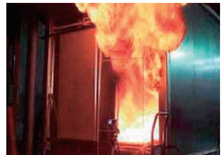
Room Corner Testing Unit (ISO 9705)
