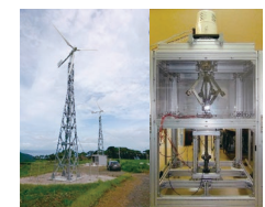
Monitoring of output power from multiple small wind turbines, and a prototype of a flywheel energy storage system
