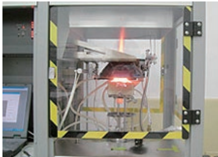
Cone Calorimeter Testing Device (ISO 5660)
