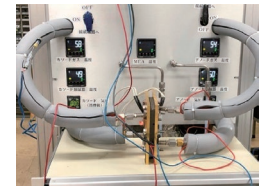
Polymer electrolyte membrane fuel cell and automatic humidity control system for supply air
