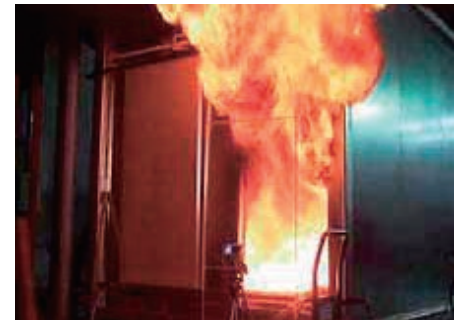
Room Corner Testing Unit (ISO 9705)
