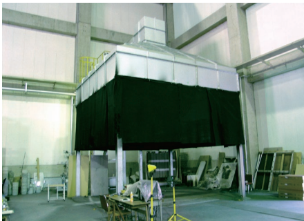
Calorimetry Hoods (5 m × 5 m)
