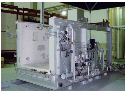
Structural Fire Testing Furnace (Medium scale)
