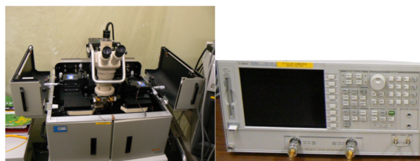
Fig. 2. Analog integrated circuit chip analysis facility. (Left: Voltage and current detection section, Right: Measurement analysis section)
