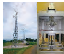
Monitoring of output power from multiple small wind turbines, and a prototype of a flywheel energy storage system
