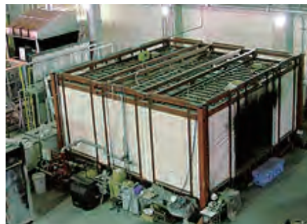
Full-Scale Compartment for Fire Experiment (with Water Pump)
