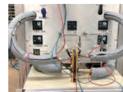
Polymer electrolyte membrane fuel cell and automatic humidity control system for supply air
