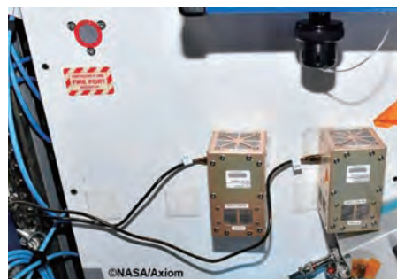
Figure 2. The photocatalytic air purification device experiment
