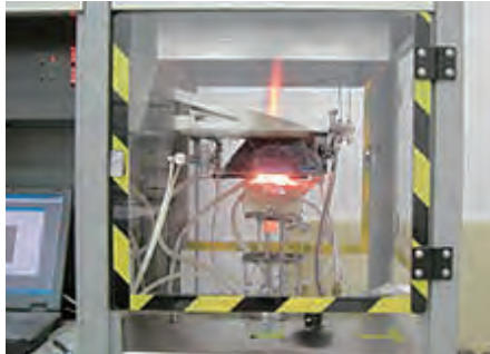
Cone Calorimeter Testing Device (ISO 5660)
