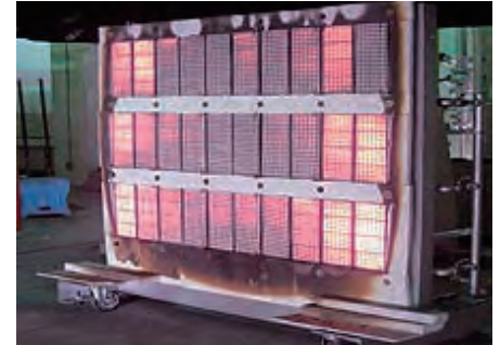
ICAL Testing Unit (Heat Radiation Panel)
