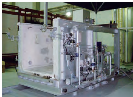
Structural Fire Testing Furnace (Medium scale)
