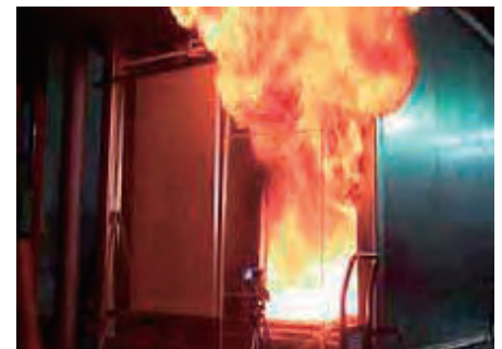
Room Corner Testing Unit (ISO 9705)
