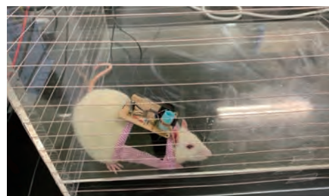
Fig. 1 Wireless power transmission to an implantable momentum meter
