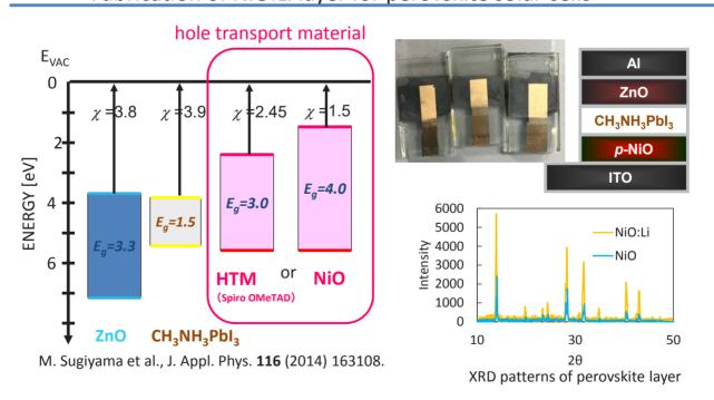
NiO:Li was used for *p* type electrode on perovskite solar cells instead of the organic material. As a result, the crystallization of the perovskite layer improved and the conversion efficiency of perovskite solar cell improved.
