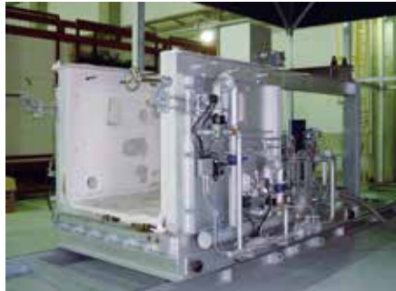
Structural Fire Testing Furnace (Medium scale)
