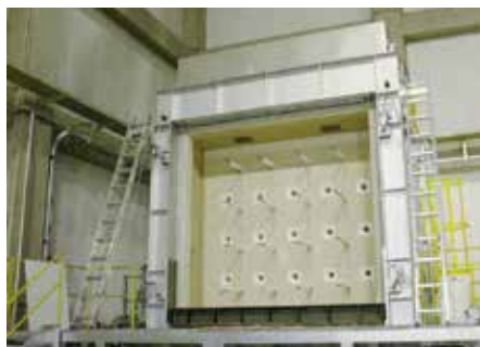
Structural Fire Testing Furnace (Large scale, for Walls)
