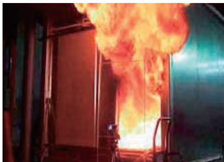
Room Corner Testing Unit (ISO 9705)
