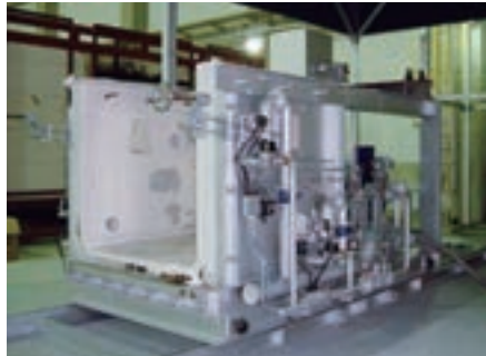
Structural Fire Testing Furnace (Medium scale)
