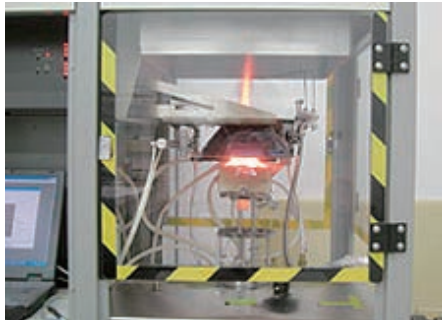
Cone Calorimeter Testing Device (ISO 5660)
