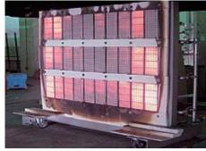
ICAL Testing Unit (Heat Radiation Panel)
