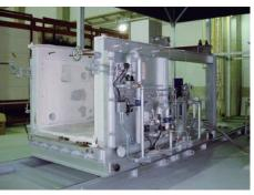
Structural Fire Testing Furnace (Medium scale)
