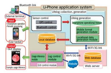
Fig.2 Li-Phone system configuration
