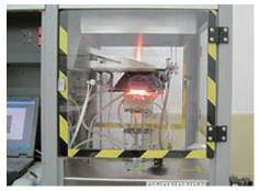
Cone Calorimeter Testing Device (ISO 5660)
