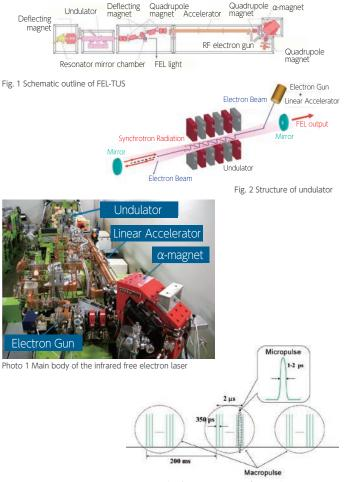
Fig. 3 Pulse time structure of FEL-TUS output
