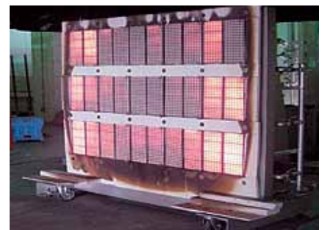
ICAL Testing Unit (Heat Radiation Panel)
