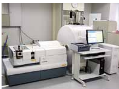
Fig. 1 Fourier Transform Ion Cyclotron Resonance Mass Spectrometer (FT-MS) (Registration No. 1077)
