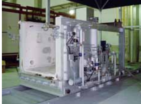
Structural Fire Testing Furnace (Medium scale)
