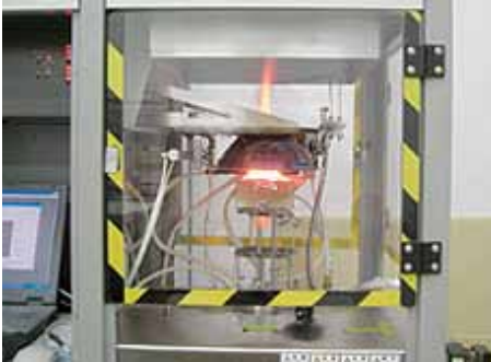
Cone Calorimeter Testing Device (ISO 5660)
