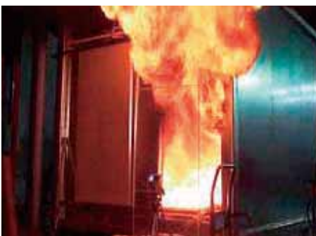
Room Corner Testing Unit (ISO 9705)
